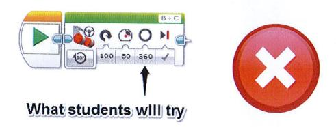
This occurs because the **Move Steering** block is designed to control the *wheel* of the robot, not the whole robot. If we observe just the wheel, we will find that it does in fact turn exactly 360 degrees, just as it was told to do. The angle turned by the robot however is dependent on a few different conditions such as the size of the wheels and the distance between the wheels.
