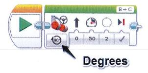
**Drive Forward 2 seconds**. How far the robot travels will be dependent on the power level chosen. Two seconds forward at 20% power will travel a different distance than two seconds forward at 100% power.
